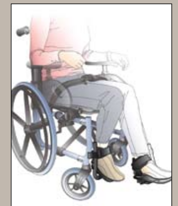
Corrected foot position with Ankle Huggers® and Adjustable Angle Footplates
