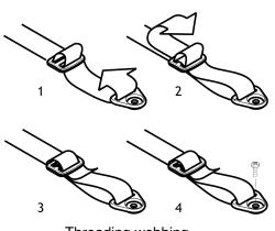
Threading webbing through the end-fitting
