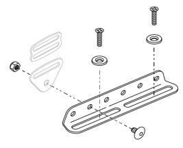
With Metal Flat-Mount™ End-Fitting, using Seat Mounting Bracket M6 x 10mm screw
