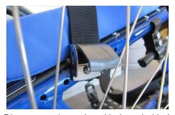
Direct mount\* on tube with threaded holes
