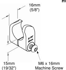
**HW310-22-A** Ø22mm (7/8") **HW310-25-A** Ø25mm (1")
