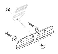
With Metal Flat-Mount™ End-Fitting, using Seat Mounting Bracket M6 X 10mm screw
