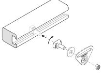
With Metal Flat-Mount™ End-Fitting using HKA10-14MM
