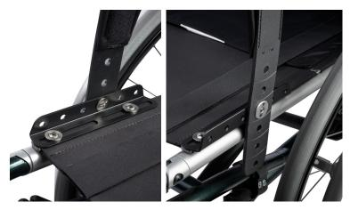
Mount on upholstery strip with Evoflex® Hip Belt, using Evoflex® M6 X 8mm screw, wave spring washer, and flange nut
