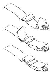
Threading webbing through the end-fitting
