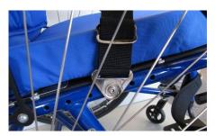
Direct mount\* on tube with threaded holes
