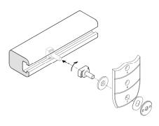
With Evoflex® Hip Belt, using HKA10-14MM stud and washer, and Evoflex® wave spring washer and flange nut
