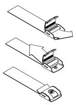
Threading webbing through the end-fitting
