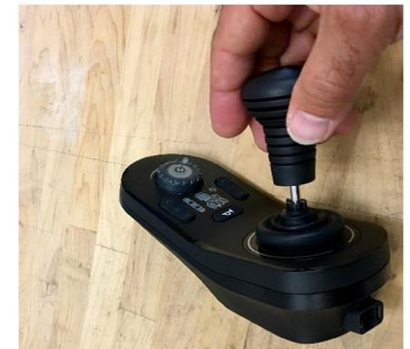
**Step 4:** Press and twist handle down fully onto stem, and allow to dry 1 hour
